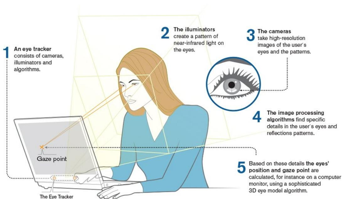
**Figure 1.** Illustration of the eye tracking process (© Tobiiipro.com)
