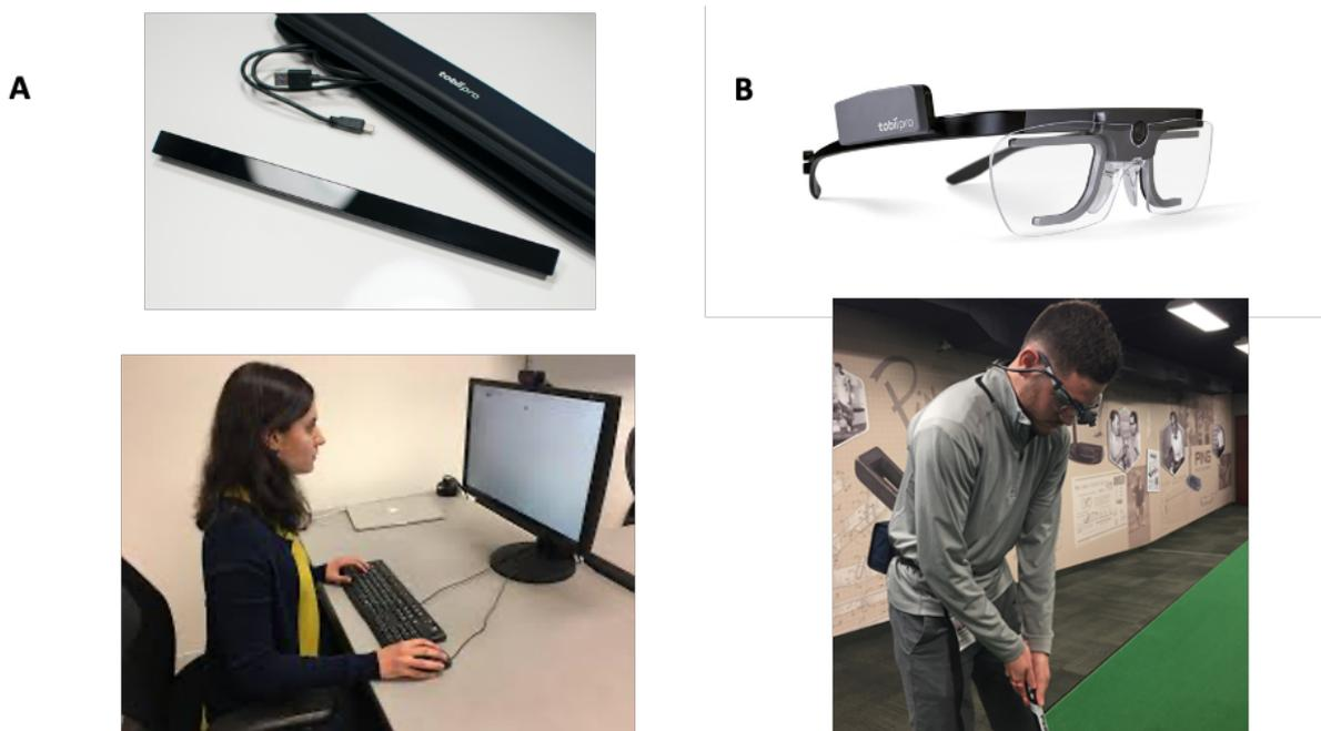
**Figure 2.** Images of the fixed (left) and wearable (right) eye trackers used in the School of Psychology. The eye tracker in panel A is the Tobii X3 120. In the lower panel, the X3 120 is attached to the bottom of the computer monitor as a participant performs a task. Panel B depicts the Tobii Glasses 2; in the lower panel, a participant wears the glasses while practicing golf.
